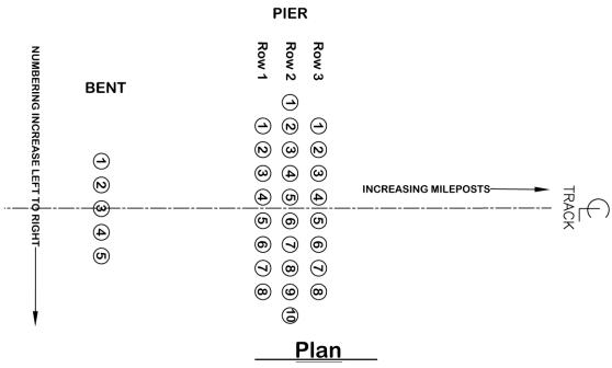
Typical Bent and Pile Pier
